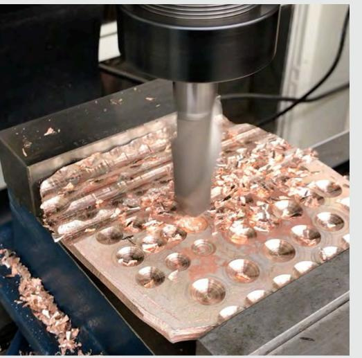
A pattern is cut into the billet with a router, drill,
