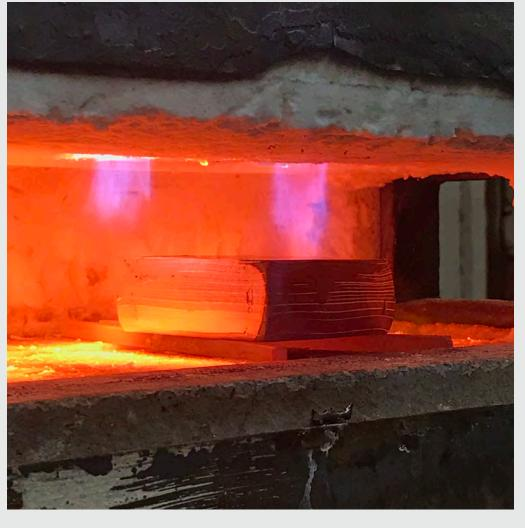
While hammering, the metal gets harder from to be annealed (heated and ready for patterning. slowly cooled) or cracks form.
