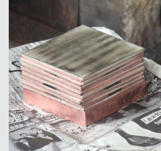
clean and dry, they are see the metal "sweating" to blow to the center of the clean, and dry. Gaps and stacked in order and then or the "flash" between layers plate. Once cool, the edges are contamination can cause pressed together between as a liquid alloy forms, fusing trimmed and inspected for any make forging it easier. plates.
